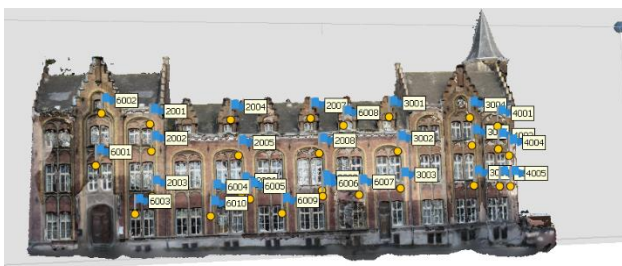
Figuur 7: spreiding GCP's over studieobject
